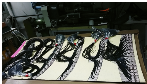
Figure 3.2: Assembly of the pressure taps in the sail
