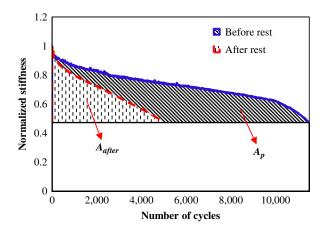
**FIG. 5**Fatigue life extension ratio index.
