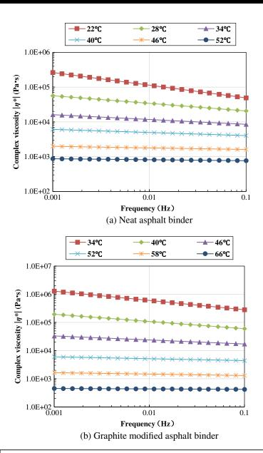
temperature was fitted in Fig. 12. The near-Newtonian transition temperatures for neat asphalt binder and graphite-modified binder is 38°C and 50°C, respectively. Based on the capillary theory to explain heating to heal in asphalt mixtures proposed in this study, the critical temperatures for neat AC and CAC to start healing are 38°C and 50°C, respectively.
