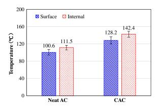
mixture specimens are about 10°C higher than the surface temperatures. This is possibly due to the fast heat dissipation on the surface. It is notable that binder at this temperature, after 120 s of heating, will be flowable and lose its bonding capability and eventually may even have negative effects on the healing level and cause binder drainage issues.
