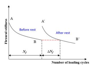
where  $N_f$  is the fatigue life of specimens before healing; and  $\Delta N_f$  is the loading cycles when the stiffness of the healed specimens reaches the 50 % stiffness of unhealed specimens, which means the extended fatigue life.
