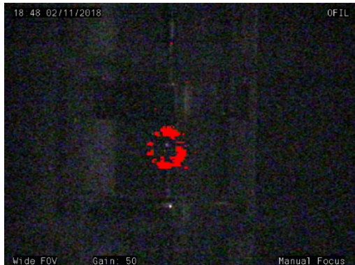
Fig. 18. The UV measurement by the corona camera showing the corona ring around the needle tip recorded at 18.5 kV_{dc} .
