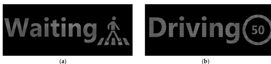
Figure 3. (a) Image presented on the eHMI when the approaching car stopped for the pedestrian, (b) Image presented on the eHMI when the approaching car did not stop for the pedestrian.
