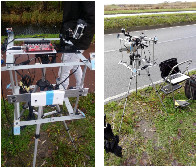
Figure 1 8-microphone array, together with the smartphone on the side and GoPro on top (Measurement Series 1).
