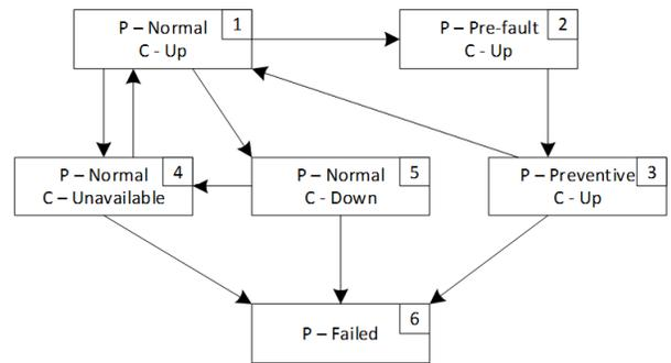
Fig. 5: State model for smart components [30]
