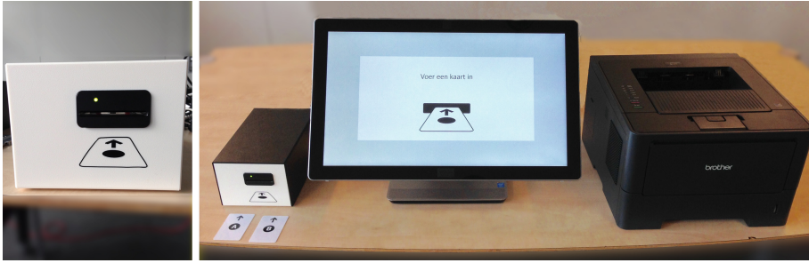
Fig. 3. Simulation of vote-printer hardware configuration; card reader, touch screen, printer
