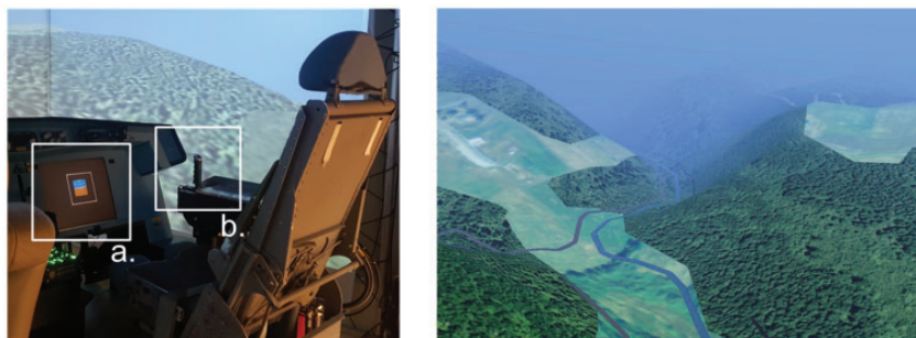
Figure 2. The simulator (left) with the AI on the head-down display (a), the sidestick on the right-hand side (b), and the head-up visual projection of two of the three screens in the background. The outside view (right), of which only the front screen is shown.
