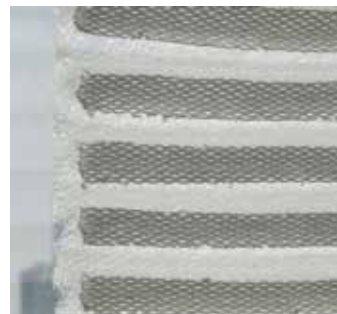
FIG. 10 Spacer textile, offset cut and stretched
