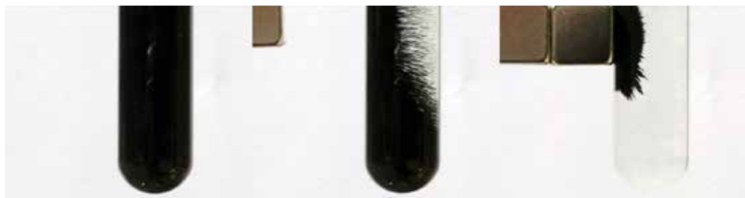
FIG. 14 Process of discoloration by means of a magnet
