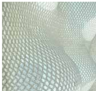
FIG. 11 Spacer textile, selectively stretched
