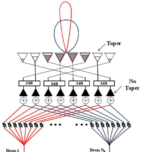
**Figure 1.** Semi-active array with phase only control.
