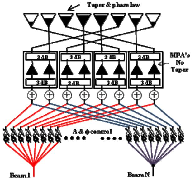
**Figure 3.** Semi-active array fed by multiport amplifiers
