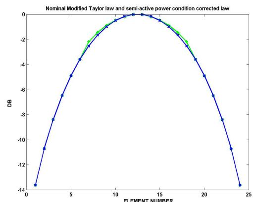
**Figure 4.** Array nominal modified Taylor law (blue) v.s. semi-active power condition corrected law (green)
