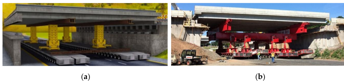
Figure 8. (a) Illustration of placing a new bridge deck with the use of an SPMT (computer-controlled platform vehicles) with jack-ups [19]; (b) placing a bridge with an SPMT during the replacement project, I-84 bridges over Marion Avenue in Southington, US [20].
