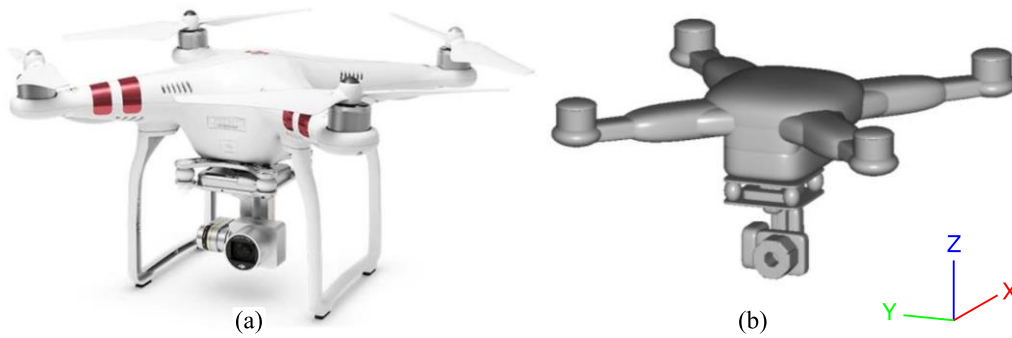
Figure 1. UAS model for impact modelling: (a) a real-world system and (b) DJI Phantom III Standard multibody system model developed in MADYMO by the author. 9 The two landing skids are neglected in the model since they are not in contact with the human head in impact cases that are investigated.
