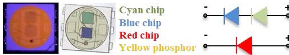
Fig. 3. A full-spectrum white LED package.
