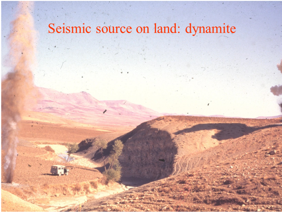
Figure 1.2: Dynamite explosion during a seismic survey. Note that the picture was taken in the 1950s, currently the safety standards are much higher and dynamite explosions are hardly visible from the surface.
