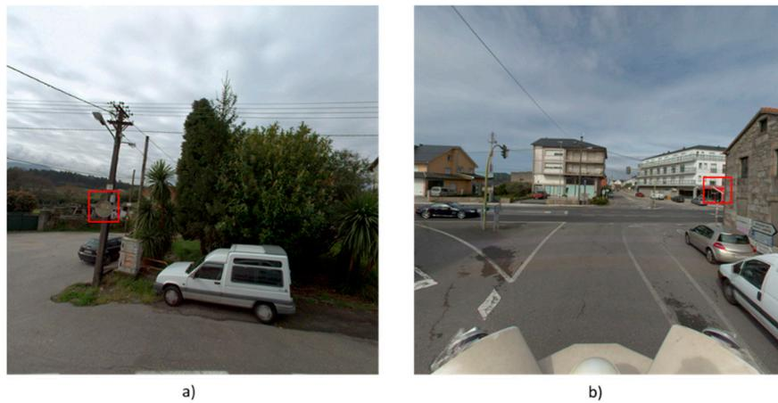
**Figure 7.** False detections (red boxes) caused by a road mirror in case study 1 (a) and by an awning in case study 2 (b).
