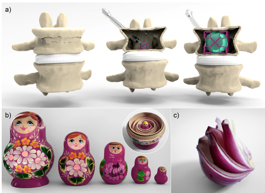
Fig. 1. a) The novel concept of deployable implants as applied to the treatment of vertebral compression fractures. With minimally invasive surgery, a deployable structure including a balloon is placed inside the fractured vertebra. Upon the inflation of the balloon, the deployable structure expands and restores the height of the vertebra. The balloon is then removed. b) Russian dolls shown from the front and top views. c) An onion also consists of different layers. (For interpretation of the references to colour in this figure legend, the reader is referred to the web version of this article.)
