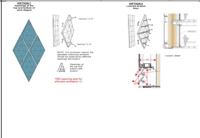
c Climate principle of the atrium and second skin. Openings of 20 m<sup>2</sup> low and high in the atrium will keep the temperature in summer close to outside temperature.
