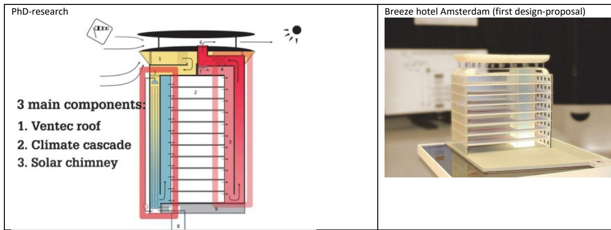
Figure 3.1.11: Earth, wind & fire research (Bronsema 2013), moderate climate, buoyancy/sun/wind/cold vapour (12 °C) to induce a vertical air flow, clean the air and provide cooling without producing a high humidity level. Mixed-mode, low air pressure building with a very high degree of natural ventilation.
