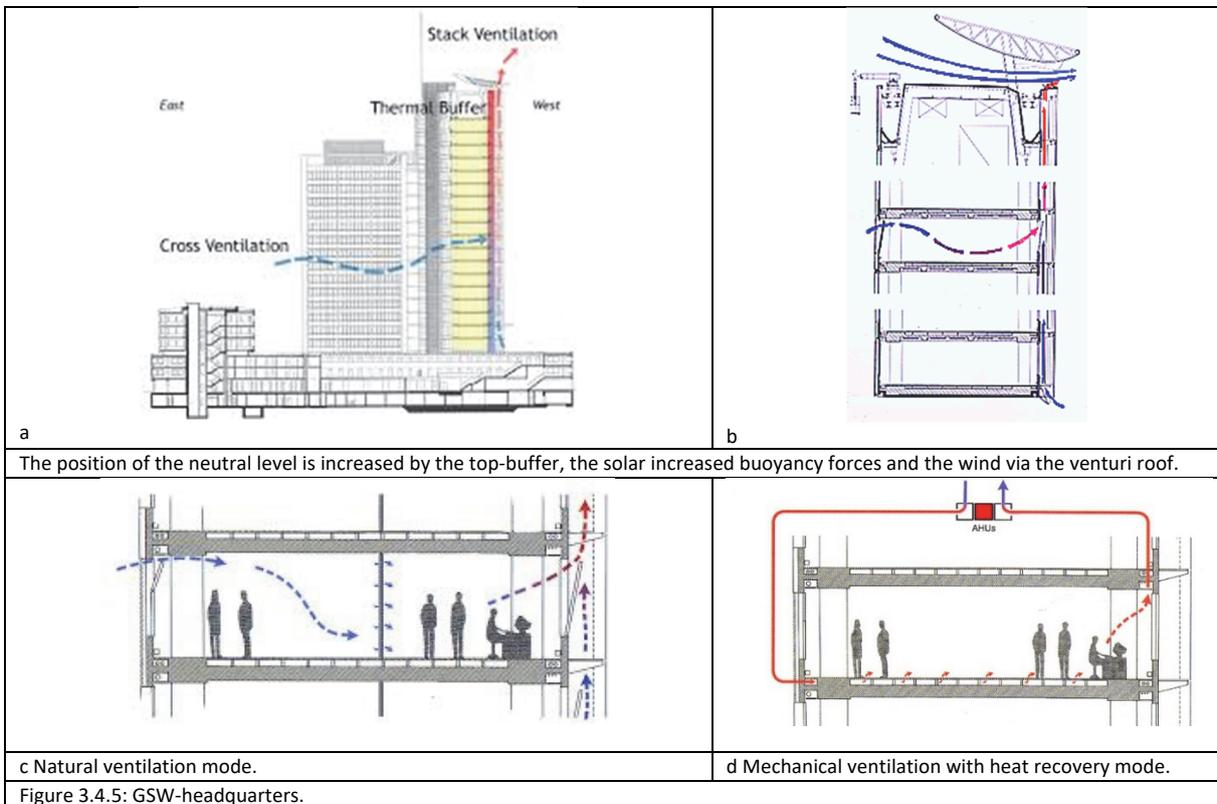
This building is a mixed mode building, in winter and summer a mechanical system can take over the climate control. The top of the façade chimney is increased to prevent reverse flows.
