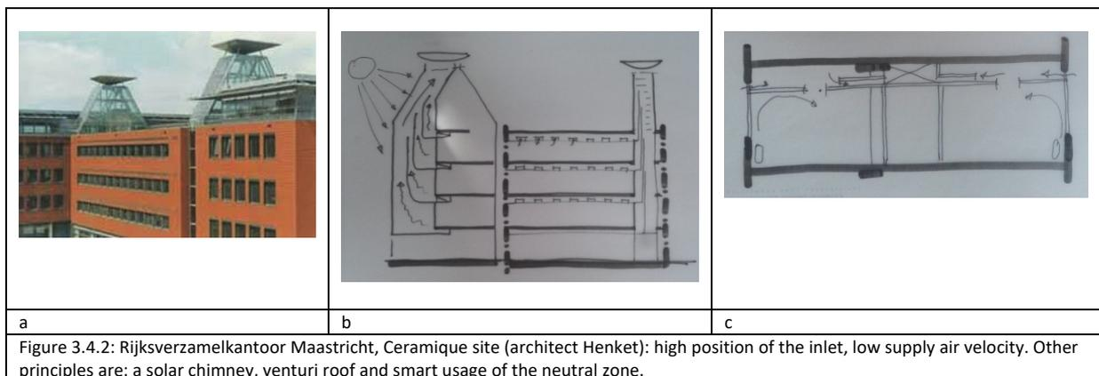
Figure 3.4.2: Rijksverzamelkantoor Maastricht, Ceramique site (architect Henket): high position of the inlet, low supply air velocity. Other principles are: a solar chimney, venturi roof and smart usage of the neutral zone.
