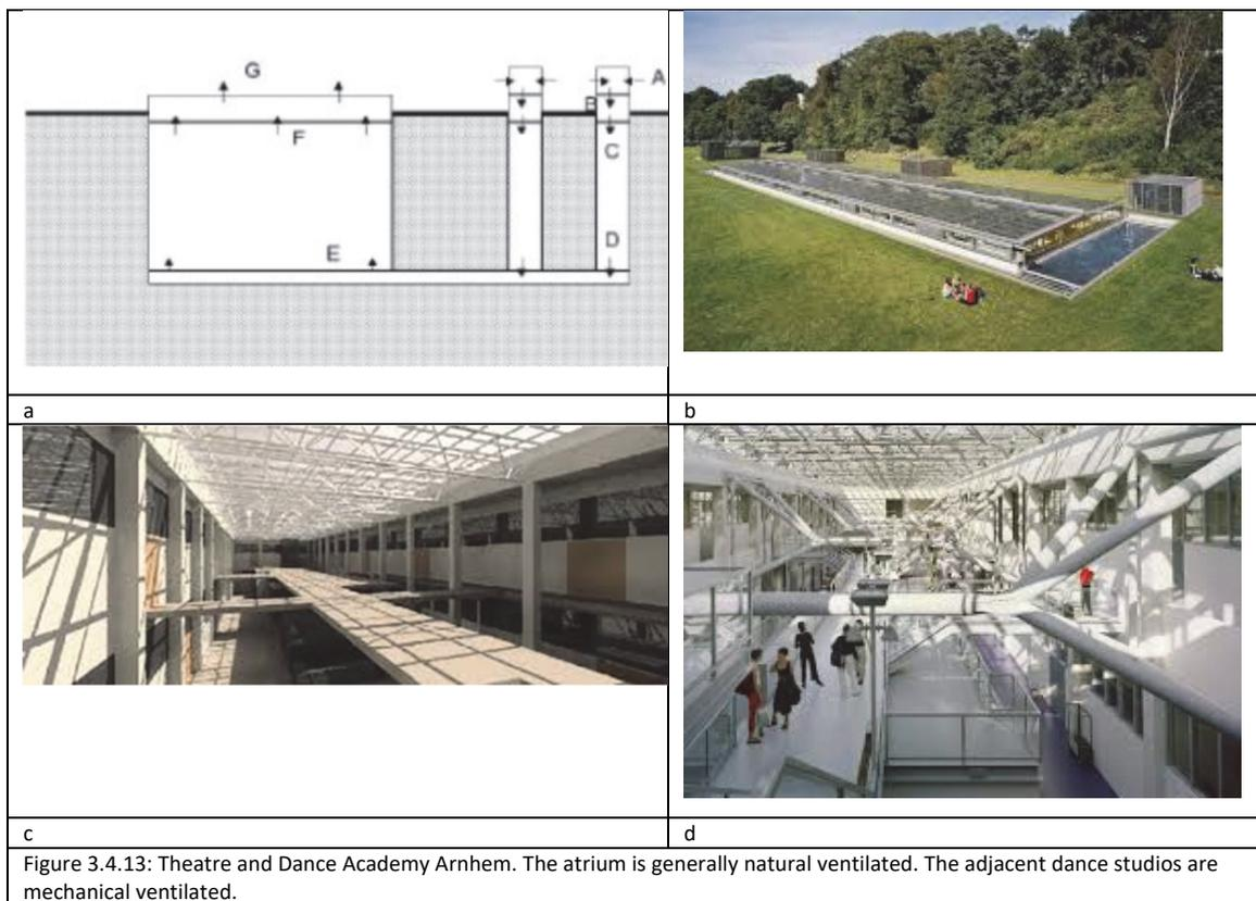
**Air supply via a ground-duct, ducts in the façade and exhaust via an atrium with chimney**
