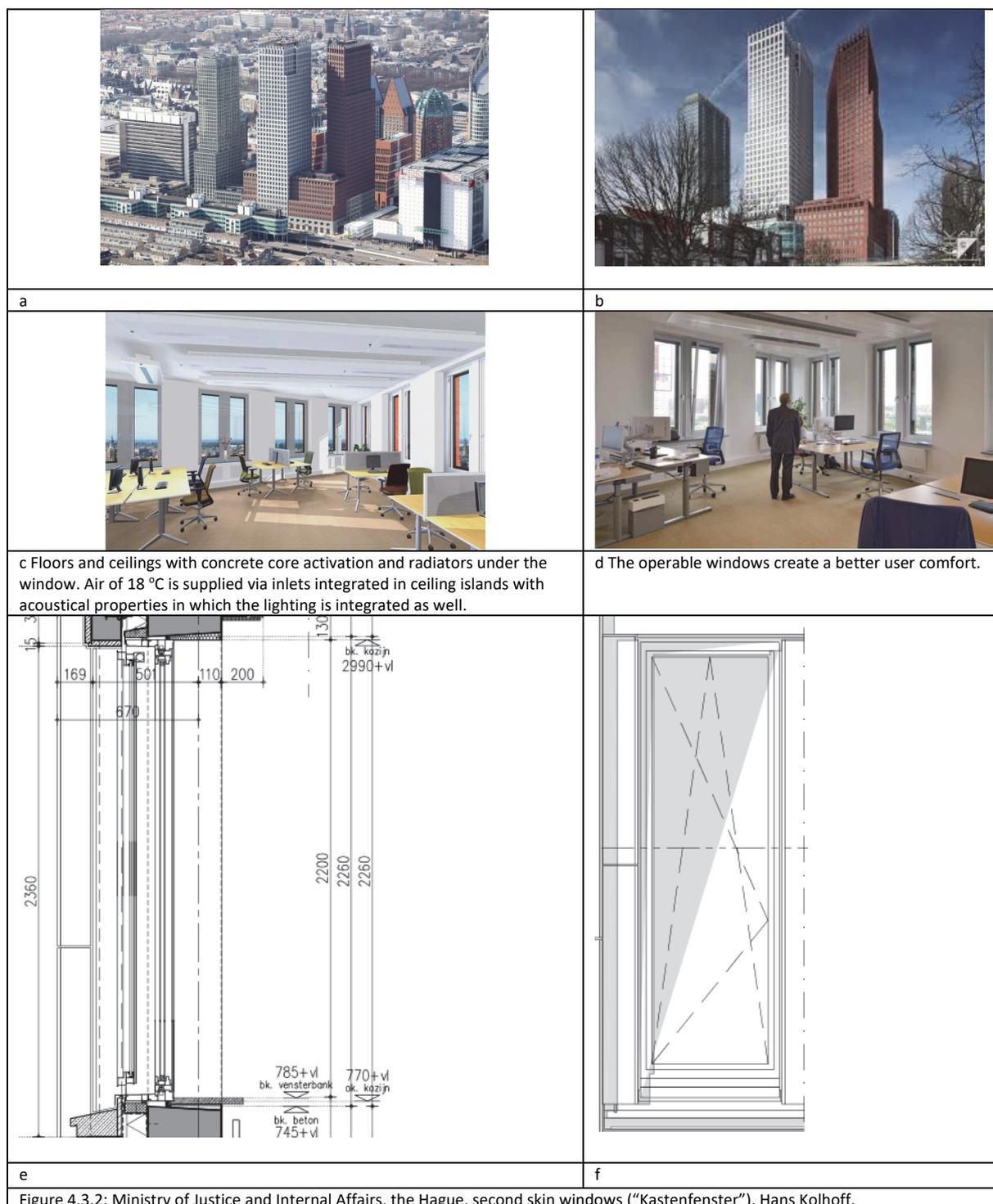
The tilt and turn windows are appreciated by the users and the fresh air supply proved to have a high cooling effect (there is always much wind around high rise buildings) as well. In fact it is a low tech option, with a minimum of control.
