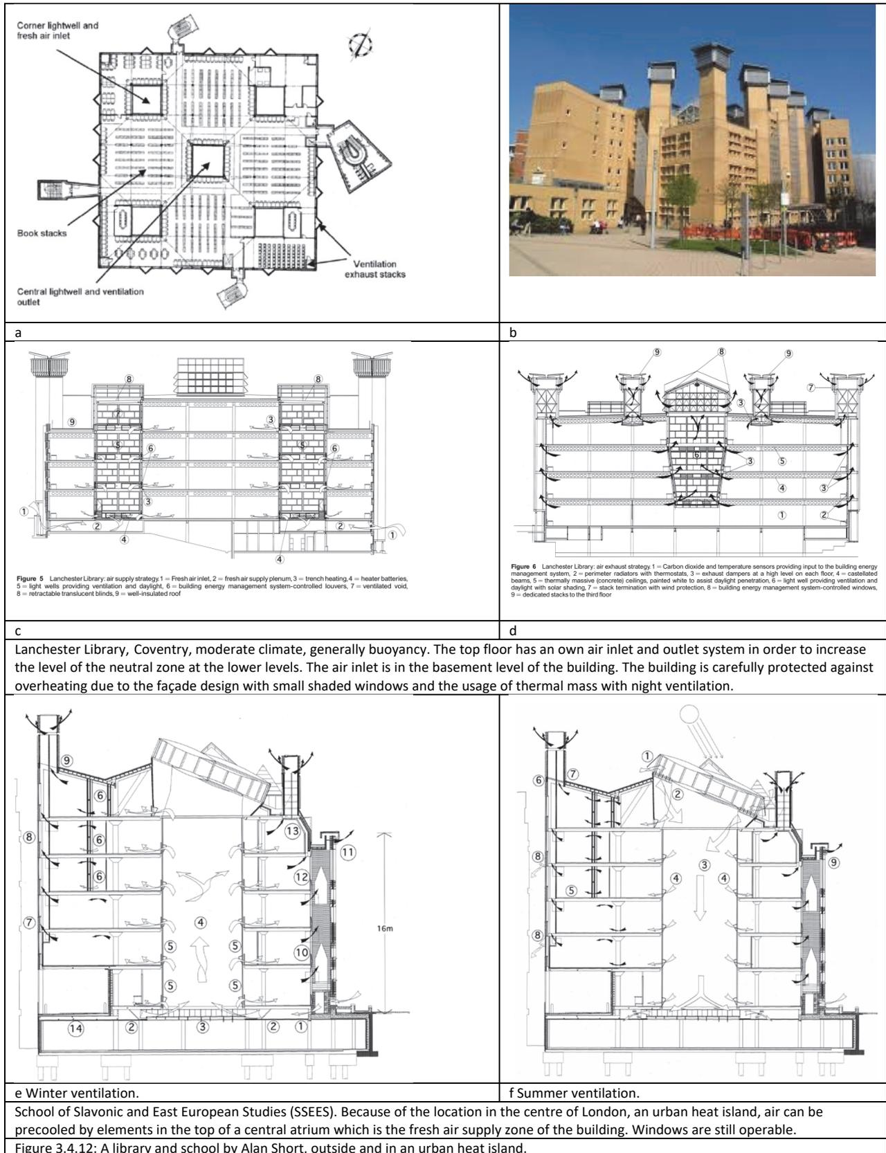
**Air supply via a shaft in the ground, supply via the ground and exhaust via the atrium-top**
