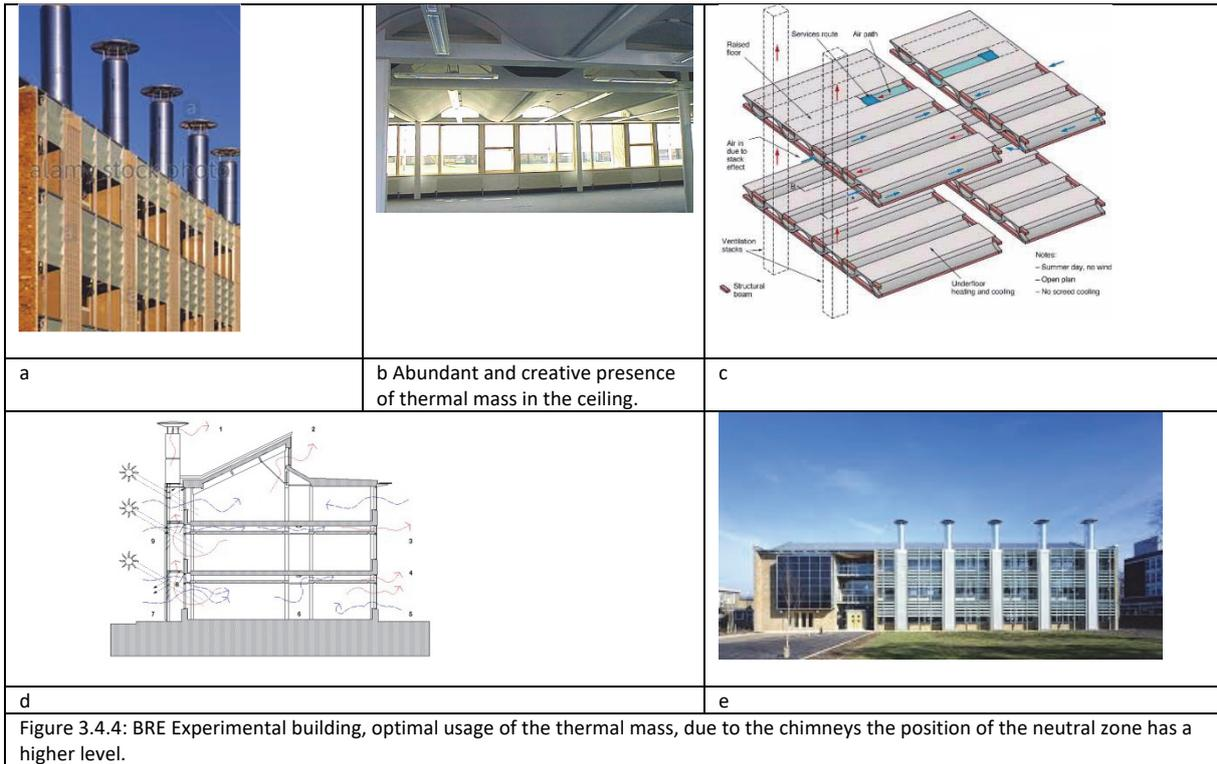
**Air supply via windows in the façade and exhaust via a shaft in the façade**
