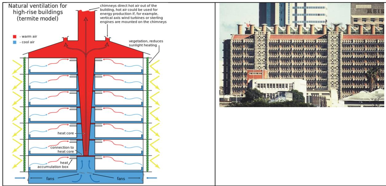
Figure 3.4.10: Eastgate Centre Harare, Mick Pierce (1996) in a hot and humid climate, air flow model inspired on the flow in a termite hill during the night, generally buoyancy. In reality the direction of air flows in termite hills reverses between day and night (King, 2015).
