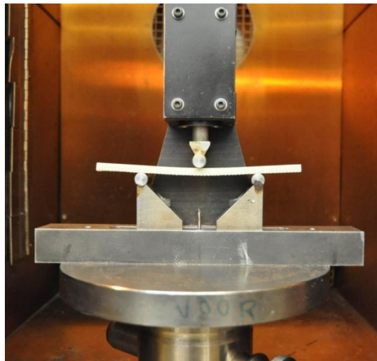
Figure 3. Flexural test device.
