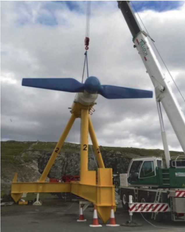
Figure 2. Nova M100 tidal turbine (Source: ©Nova Innovation).
