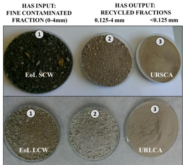
**Fig. 4.** (1) HAS input. (2&3) HAS recycled fractions.
