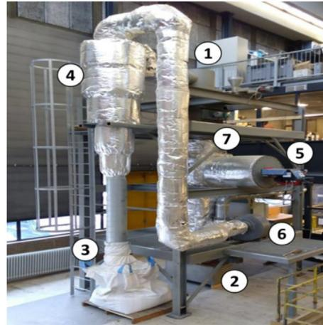
**Fig. 2.** Diagram of HAS and working principles (Left). A pilot scale HAS lab setup at the Delft University of Technology (Right): 1) Aggregate feed; 2) Recycled fine particles; 3) Recycled ultrafine particles; 4) Cyclone; 5) Burner; 6) Blower; 7) Separation chamber.
