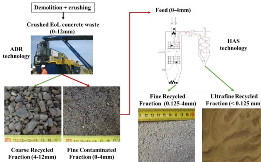
Fig. 1. Material flow in the recycling process.
