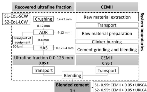
Fig. 5. System boundaries of blended cement production.
