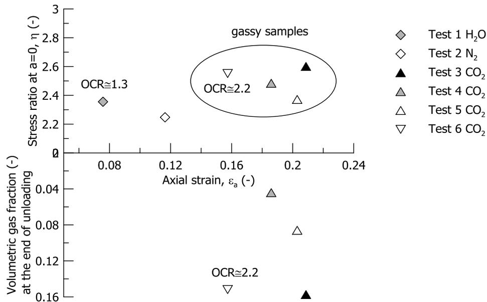
Fig. 16. Stress ratio plotted against axial strain at the onset of failure together with the volumetric gas fraction generated at the end of undrained unloading
