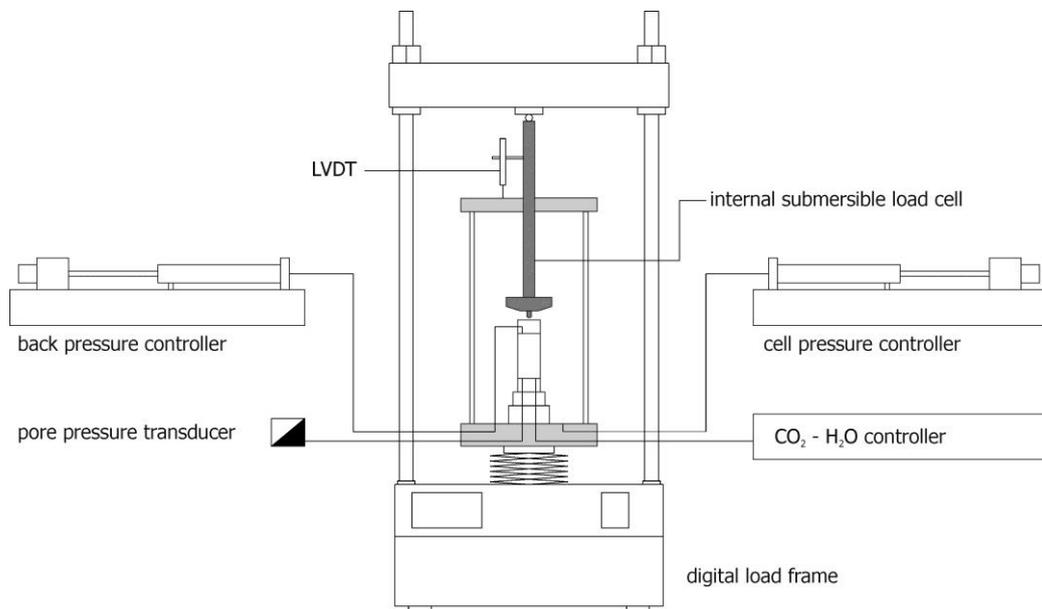
Fig. 1. Triaxial testing system including the pressure/volume controllers and the carbonated water flushing system (LVDT, linear variable differential transducer)
