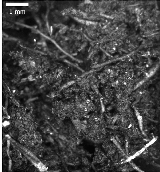
Fig. 6. Micrographs of the tested peat fabric from polarised microscopy
