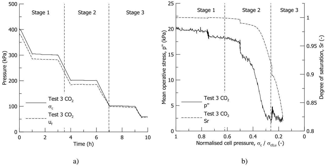
Fig. 7. Test 3 CO<sub>2</sub>: (a) cell pressure and pore fluid pressure evolution, (b) mean operative stress and degree of saturation evolution during undrained unloading
