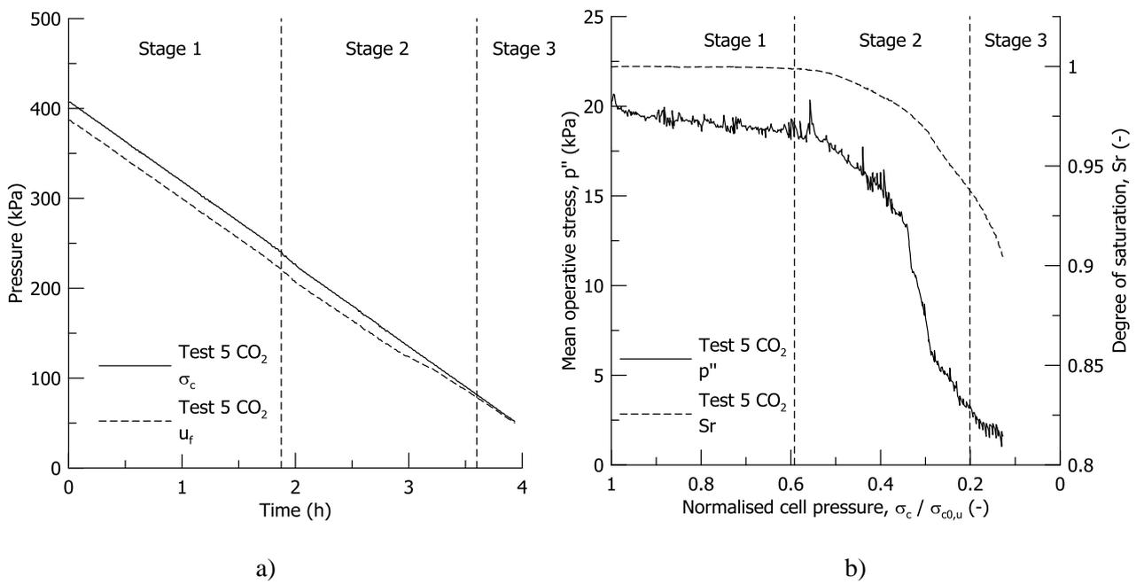
Fig. 8. Test 5 CO<sub>2</sub>: (a) cell pressure and pore fluid pressure evolution, (b) mean operative stress and degree of saturation evolution during undrained unloading
