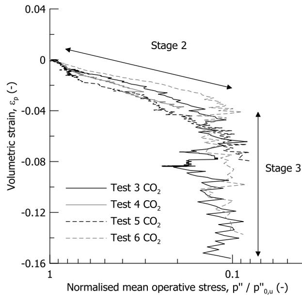
Fig. 12. Volumetric strains plotted against operative stress during undrained unloading for the gassy samples
