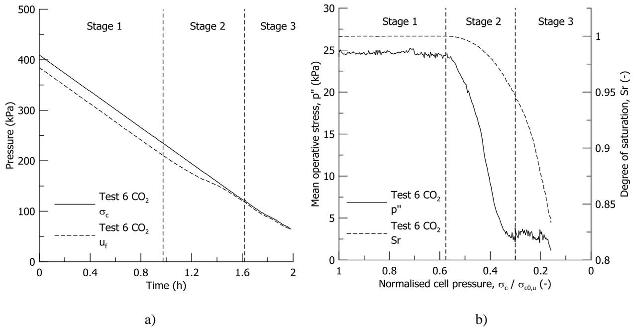
Fig. 9. Test 6 CO<sub>2</sub>: (a) cell pressure and pore fluid pressure evolution, (b) mean operative stress and degree of saturation evolution during undrained unloading
