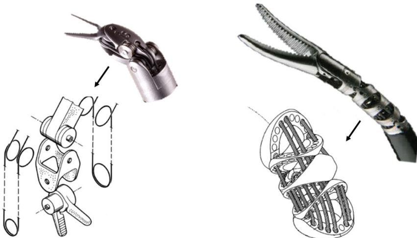
Figure 2.3: Two versions of the EndoWrist developed by Intuitive Surgical Inc. Left:  $\varnothing 8$  mm pulley mechanism (adapted with permission from [44], copyright IEEE 2005). Right:  $\varnothing 5$  mm stacked multi jointed version.
