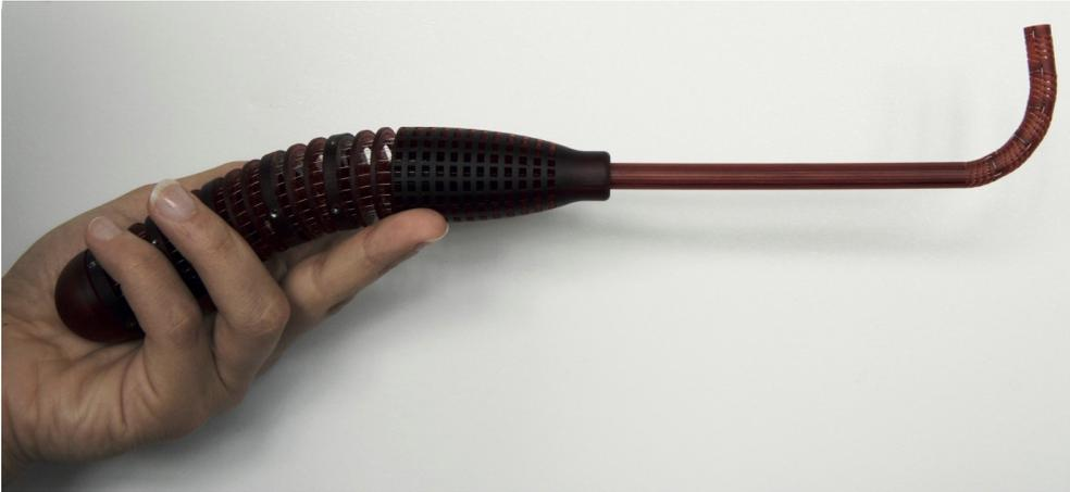
Figure 3.6: The assembled HelicoFlex prototype showing a single curve.
