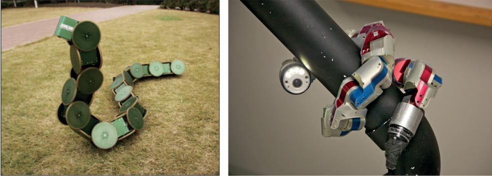
Figure 1.7: Snake-like robots. Left: ACM-R3 snake robot developed at the Tokyo Institute of Technology © [2009] IEEE [22]. Right: Uncle Sam, a snake robot developed at the Robotics Institute of Carnegie Mellon University. 'Snake robot at the Robotics institute', image by Jiuguang Wang, [www.robo.guru](http://www.robo.guru), licensed under CC BY-SA 2.0.
