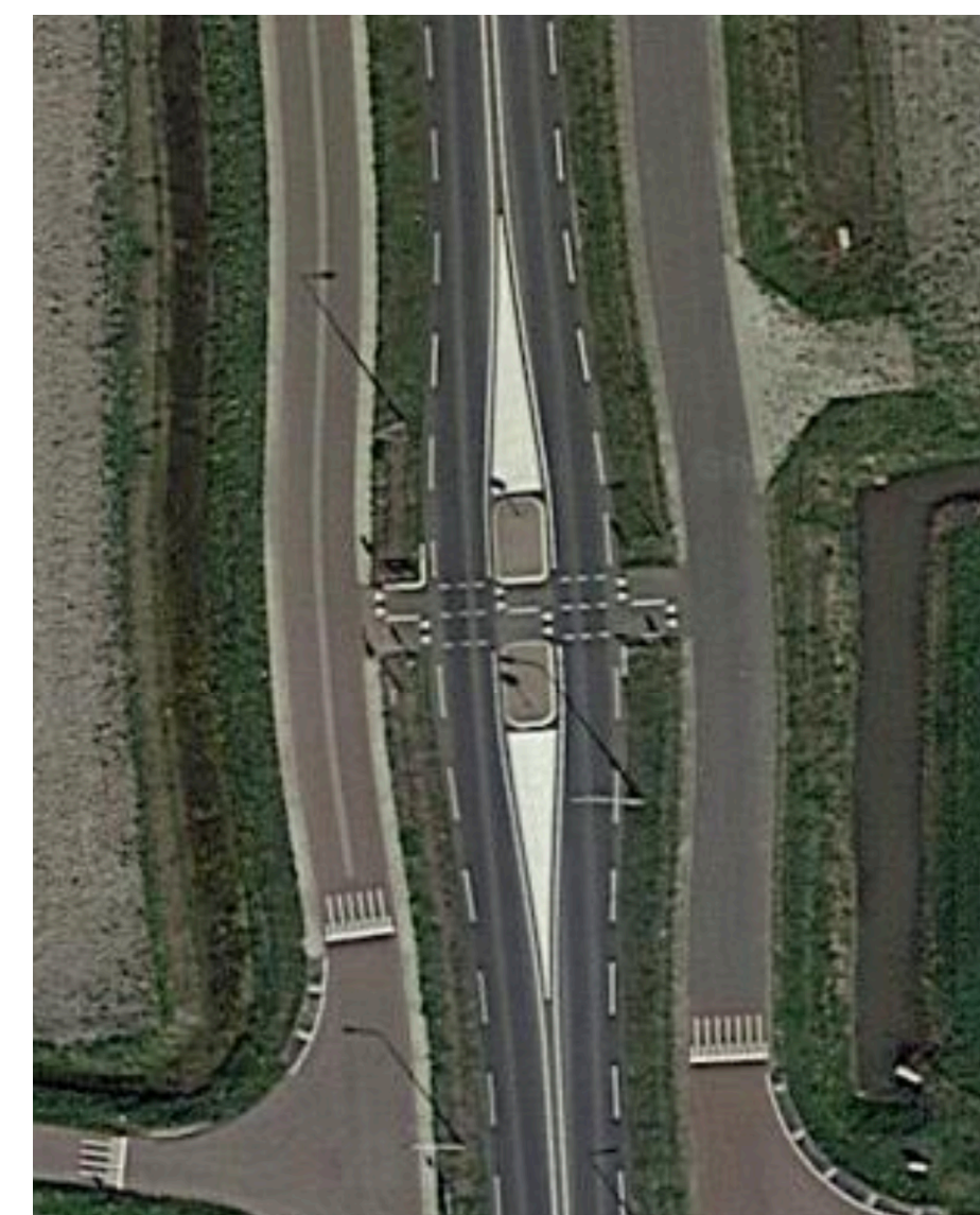
Median with crossings has too sharp curves
