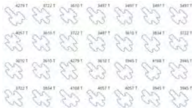
Figure 12: Excerpt of the resulting geometries and the corresponding objective values (mass)
