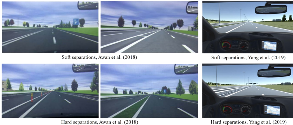
Fig. 2. Examples of hard and soft separation on managed lanes used in the literature.
