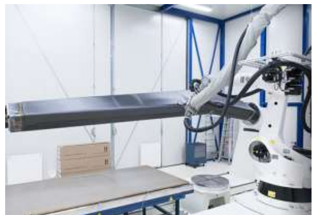
Figure 5: Flat lay-up concept for skin preforms with NLR's AFP machine (top); NLR's AFP machine placing a large thermoplastic pylon upper spar (bottom)
