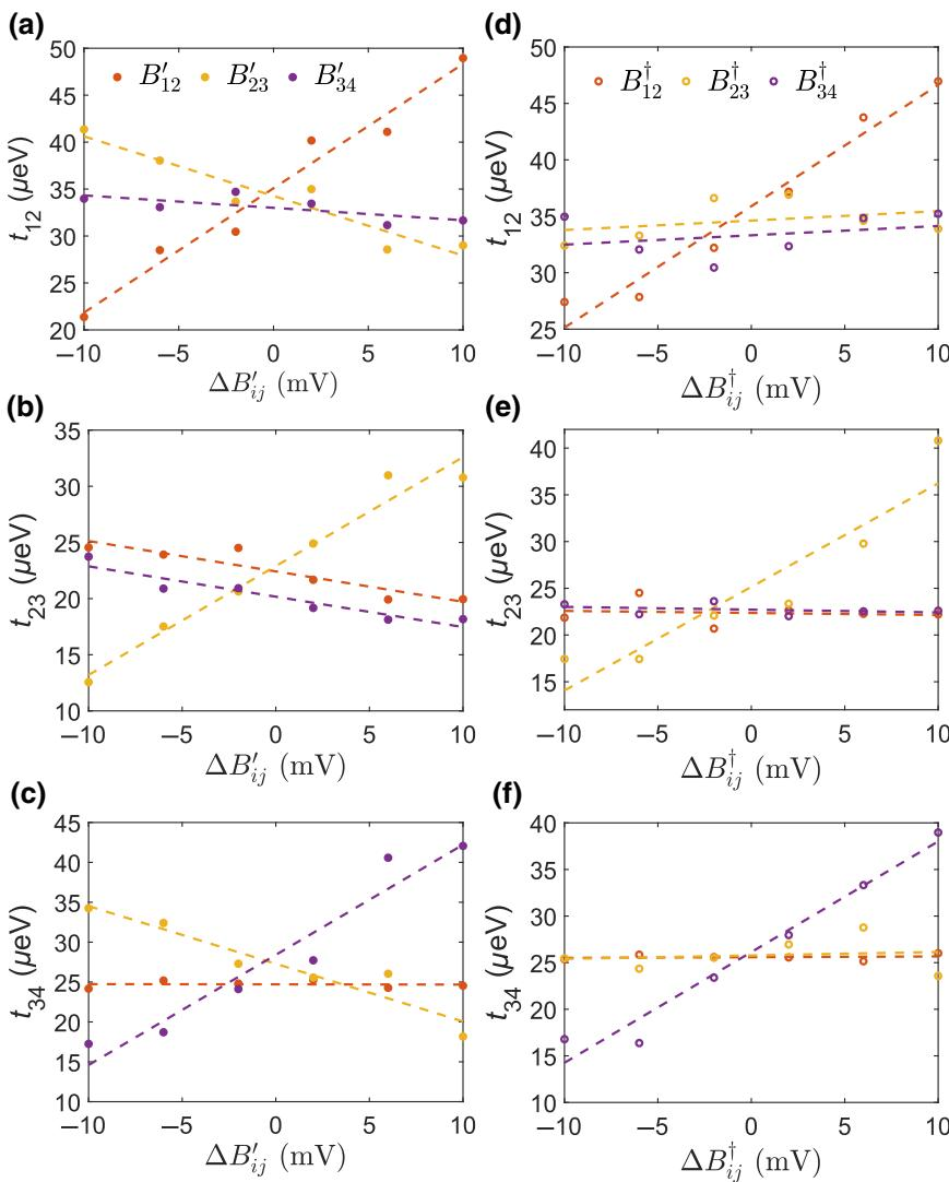
FIG. 3. (a)–(c) Measured tunnel couplings as a function of  $B'$  for (a)  $t_{23}$ , (b)  $t_{12}$ , and (c)  $t_{34}$ . Dashed lines show linear fits to the data. (d)–(f) Measured tunnel couplings as a function of  $B^\dagger$  for (d)  $t_{23}$ , (e)  $t_{12}$ , and (f)  $t_{34}$ . After calibration, each  $t_{ij}$  only depends on the corresponding  $B_{ij}^\dagger$ . Dashed lines show linear fits to the data.
