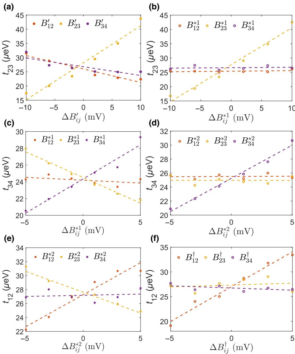
FIG. 7. Stepwise tuning and calibration of tunnel couplings:  $t_{23}$  as a function of (a)  $B'$  and (b)  $B^{*1}$ ;  $t_{34}$  as a function of (c)  $B^{*1}$  and (d)  $B^{*2}$ ;  $t_{12}$  as a function of (e)  $B^{*2}$  and (f)  $B^\dagger$ .
