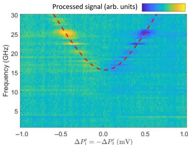
FIG. 5. Photon-assisted tunneling measurement showing the sensor signal as a function of frequency and detuning at the  $(1, 0, 1, 1)-(0, 1, 1, 1)$  interdot transition, shown after background subtraction [18]. The red dashed line is the fit of the form  $hf = \sqrt{\epsilon_{12}^2 + 4t_{12}^2}$ .
