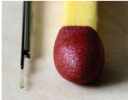
Figure 8.1. Multi-functional needle prototype containing one fiber optic, a Nitinol tube and Nitinol wires.
