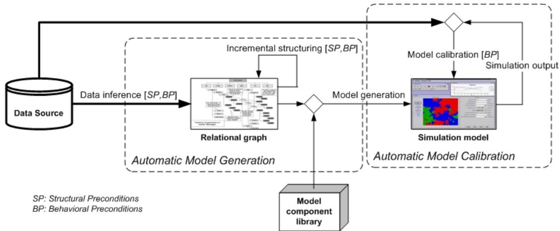
Figure 1: Component-based model generation with a data-driven approach.
