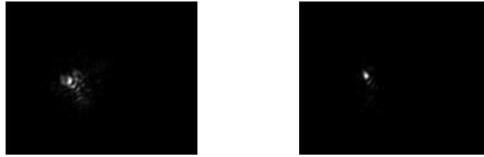
(a) External aberration generated with an aberration generator
