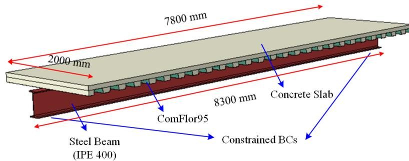
**Fig. 1:** Dimension of the composite steel-concrete girder
