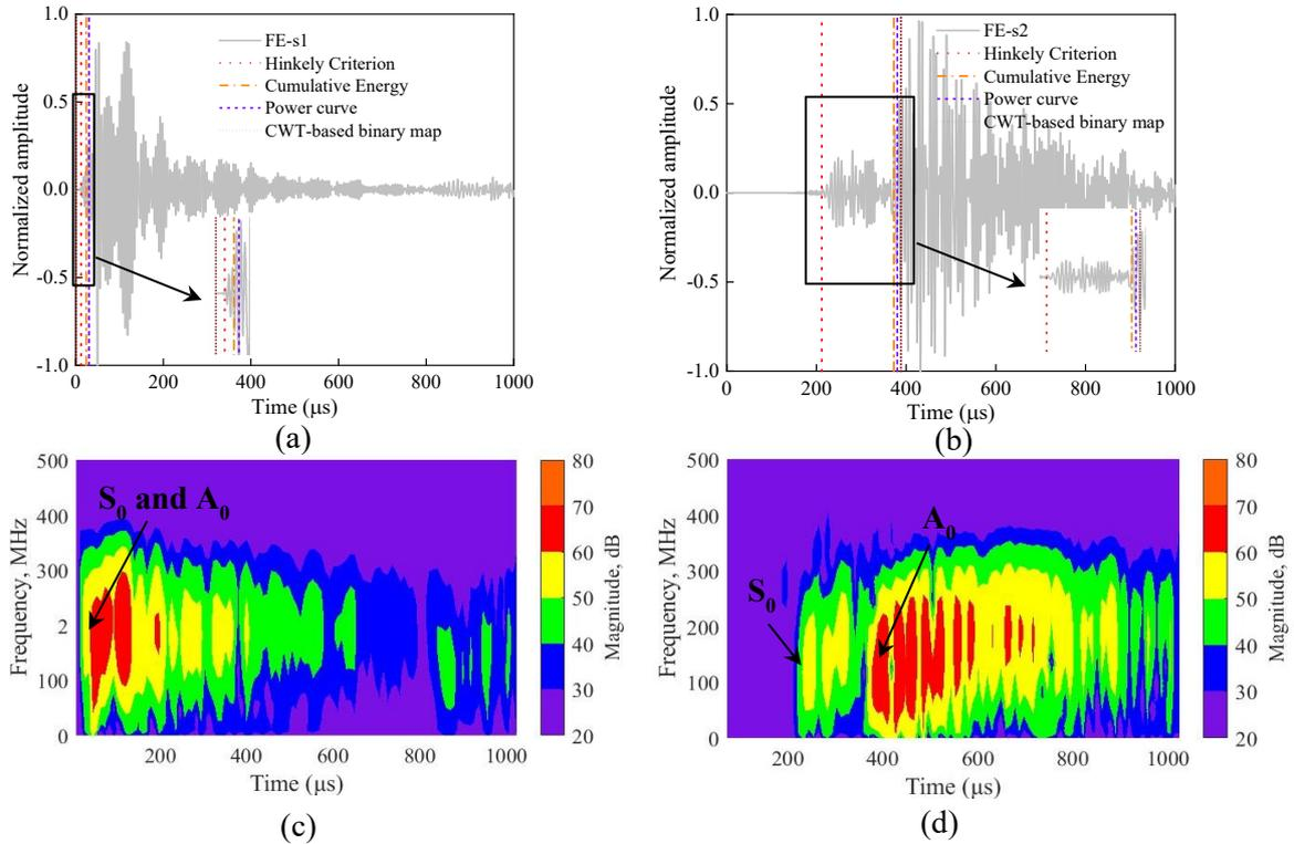
**Fig. 9:** Onset detection using selected methods of linear array obtained from FE model: signals at (a) sensor 1 and (b) sensor 2; Amplitude spectrogram of signals at (c) sensor 1 and (d) sensor 2
