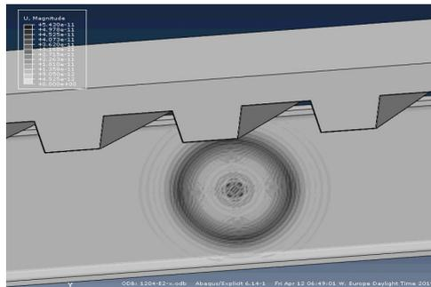
**Fig. 5:** Illustration of Lamb waves propagation in ABAQUS
