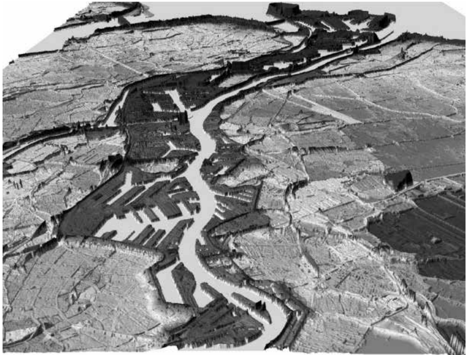
FIGURE 5.1 man-made landscape of elevated ports located outside of the primary flood protection system and deeply subsided polders (dark grey area) that are located several meters below sea level. Picture: City of Rotterdam/ TU Delft- Inge Bobbink.
