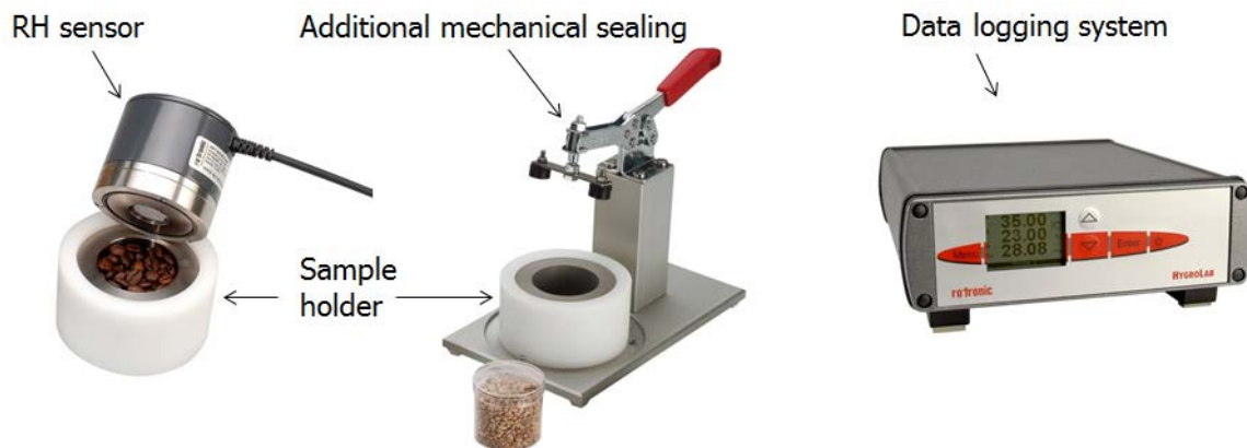
Fig. 1 Set-up for RH measurement
