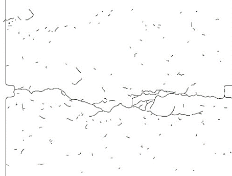
Figure 5.40 Fracture pattern for representative MSHB test on BFS cement concrete Wet (07HW04).
