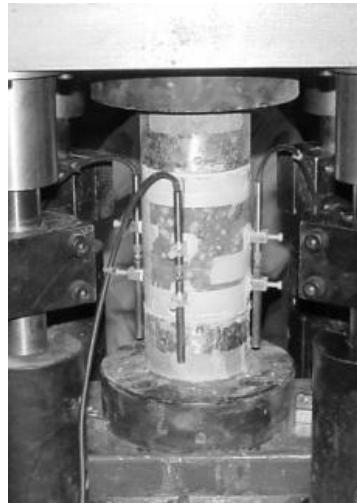
Figure 3.8 Detail of static specimen glued into set-up.
