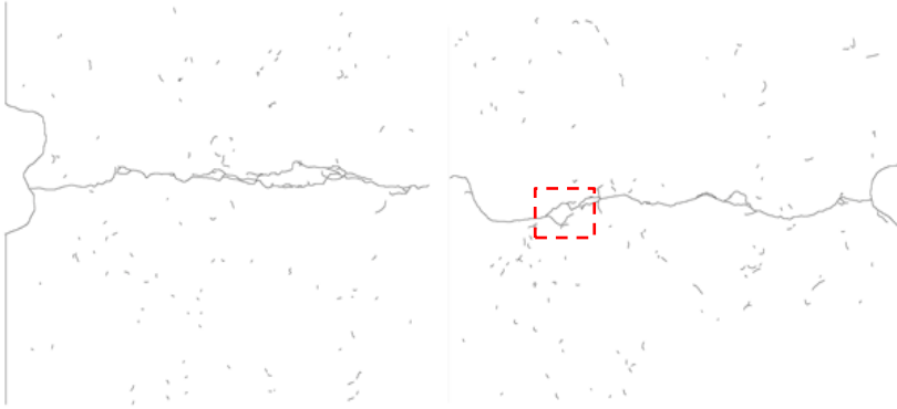
Figure 4.21 Static fracture: crack branching (test 03D2).
