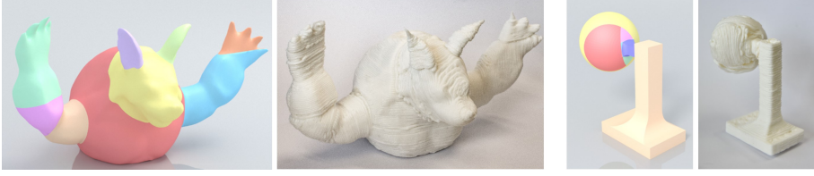
Figure 2.8: More examples that are fabricated by our RoboFDM system – (left) Armadillo and (right) Hanging-Ball without adding any supporting structure.
