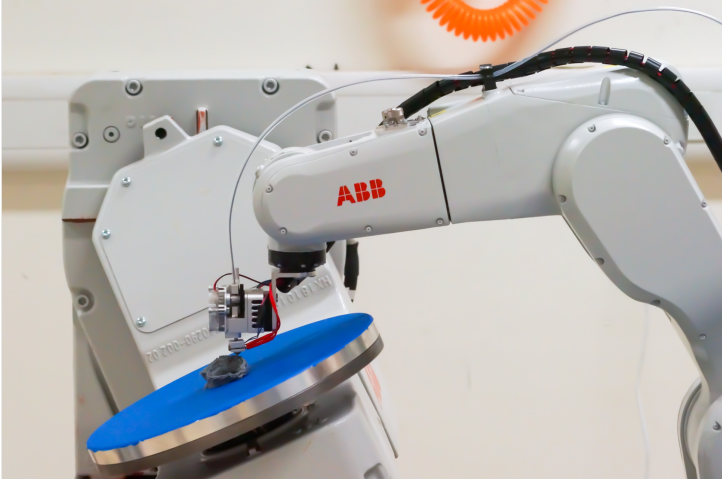
Figure 4.8: A hardware setup of robot-assisted AM system with 8-DOFs consisting of a 6-DOF ABB IRB1200-7/0.7 robotic arm and a 2-DOF IRBP A-250 tilting table.
