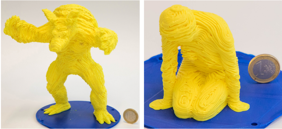
Figure 3.13: The results of our algorithm for manufacturing an Armadillo model and a Woman-Pully model by our robot-assisted AM setup.
