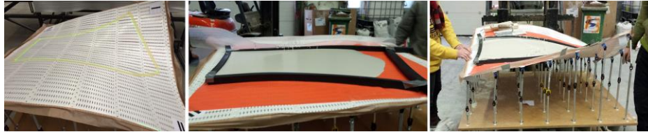
Fig. 1. Flexible mould system before and after deformation [1].
