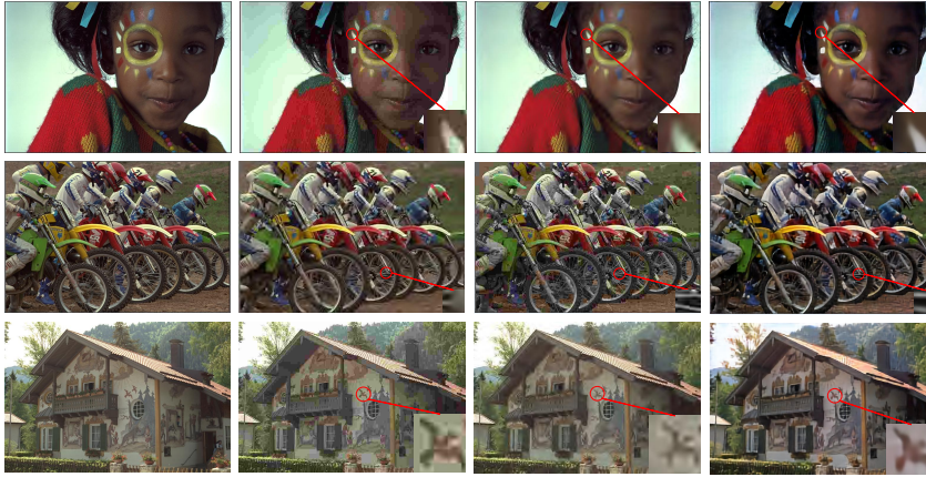
Fig. 8 Samples from Kodak dataset for visualization. Ground truth, JPEG, JPEG 2000 and Ours BGAN+ are from left to right (0.15 bit/px).
