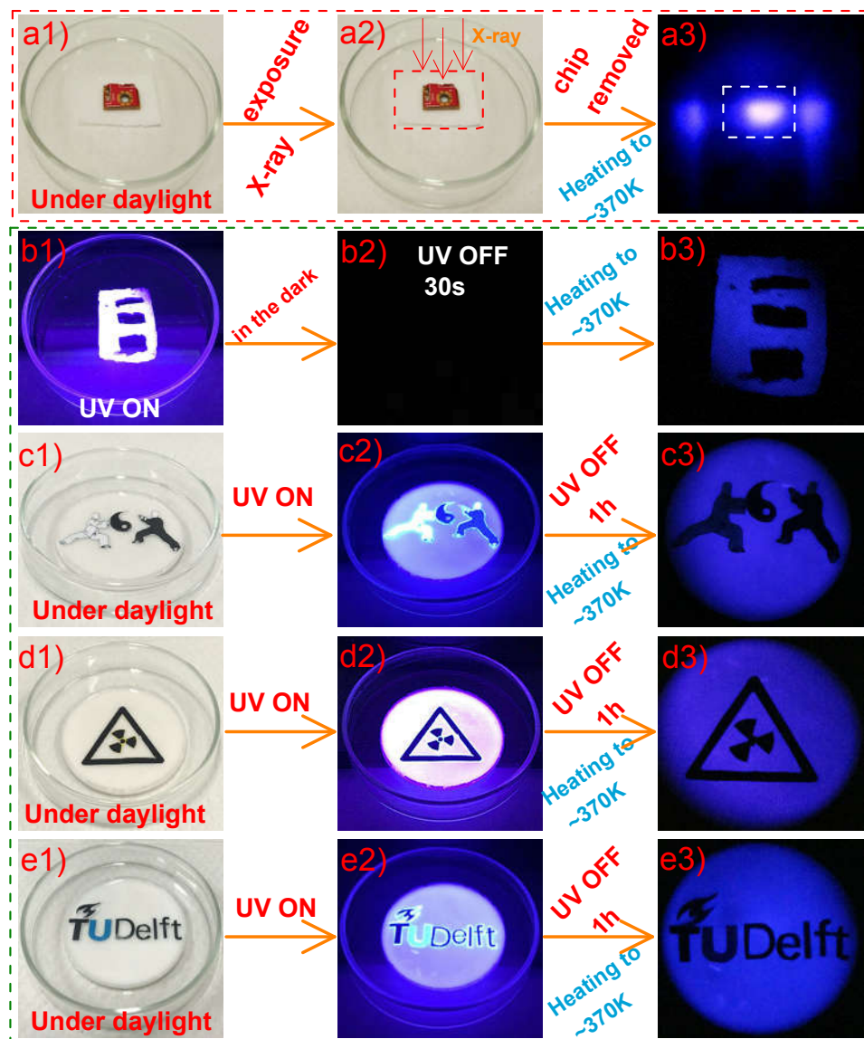
Fig. S6.29. Proof-of-concept information storage application by using \text{LiLu}_{0.5}\text{Y}_{0.5}\text{SiO}_4:0.01\text{Ce}^{3+}, 0.01\text{Sm}^{3+} phosphor dispersed in a silicone gel plate. Information storage and display of an X-ray photograph of a chip in a1)-a3), and of different logos in b1)-e3).
