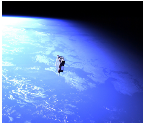
Figure 2.2: Cooperative close-proximity operations (distance of about 15 m) during the PRISMA mission (image credit: OHB-Sweden).
