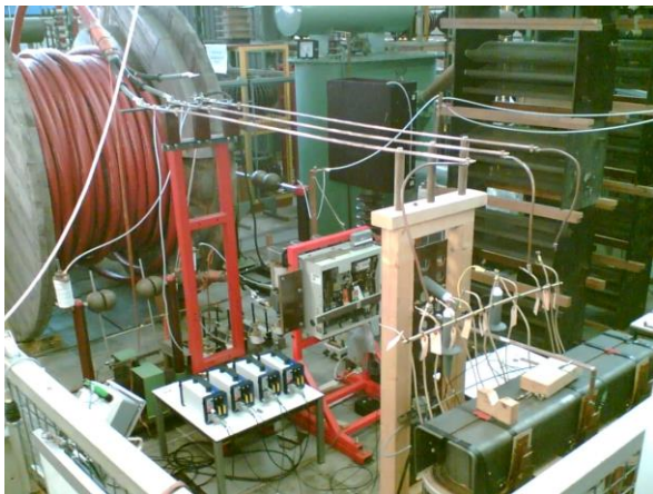
Figure 7. Transformer switching test circuit.
