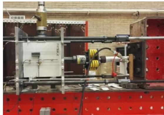
Figure 46 – Shear-compression test on the CS element masonry: (a) adopted specimen; (b) test set-up.
