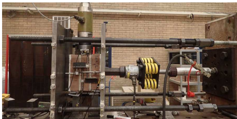
Figure 53 – Test set-up for the shear-compression test on masonry specimen.
