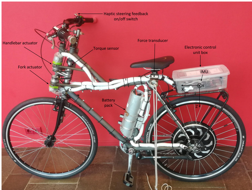
Figure 8.2: Steer-by-wire bicycle prototype with handlebar and fork actuators, sensors, pulling rope mechanism, digital controller and custom made battery pack.
