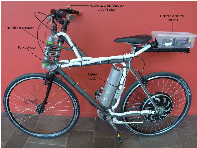
Figure 4.5: Steer-by-wire bicycle prototype with handlebar and fork actuators, sensors, digital controller and custom made battery pack.
