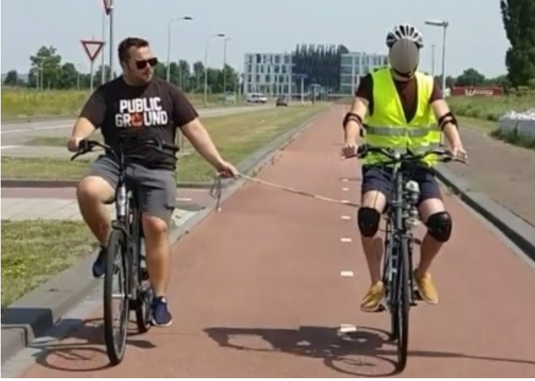
Figure 5.2: Experimental trial performed across Heertjeslaan cycling path of TU Delft; Experiment coordinator cycling next to steer-by-wire bicycle while pulling laterally the subject with a rope.
