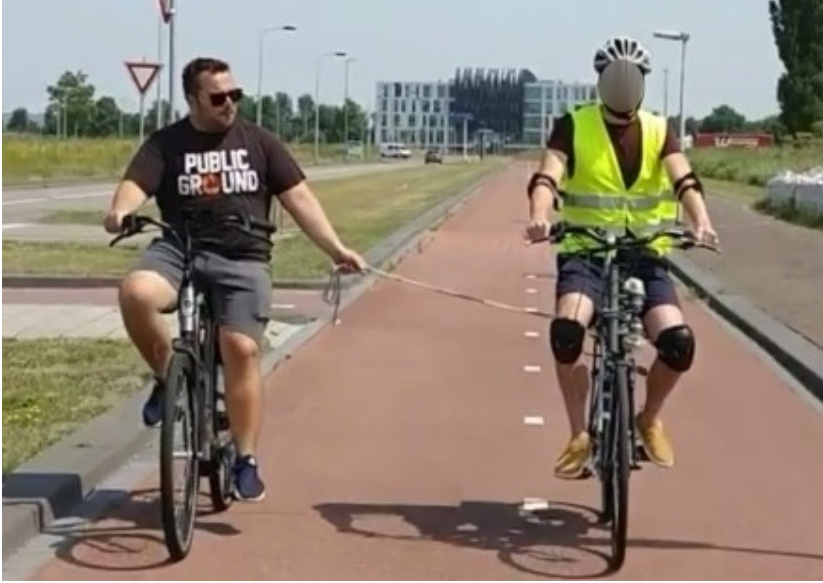
Figure 6.3: Experimental trial performed at TU Delft; The experiment coordinator (left) cycling next to the steer-by-wire bicycle (right) applies an impulsive lateral force with a rope.
