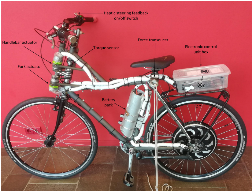
Figure 6.1: Steer-by-wire bicycle prototype with handlebar and fork actuators, sensors, pulling rope mechanism, digital controller and custom made battery pack.
