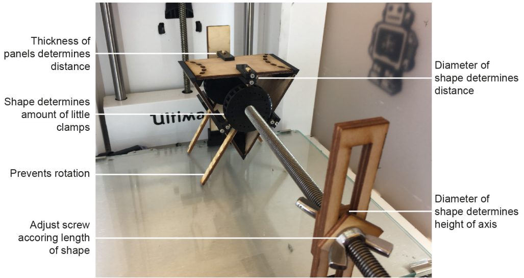
Figure 4.4. A clamp holds face panels of different widths and lengths at specific angles with corner parts on the 3D print bed. The height of the prism can be raised or lowered.
