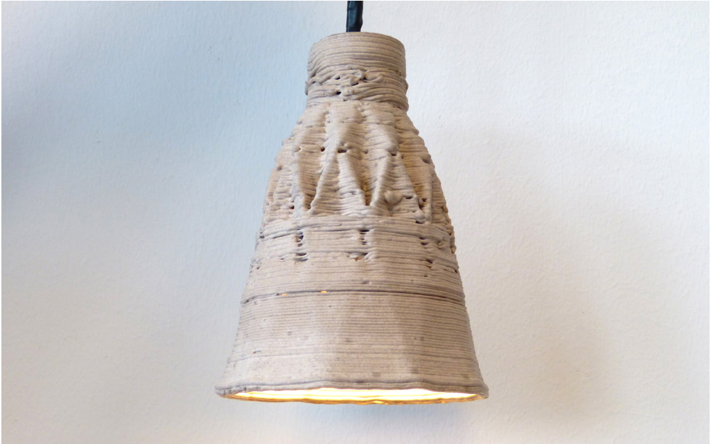
Figure 6.1. Lampshade 3D printed with a composite material from mussel shells and sugar water (design from Joost Vette)
