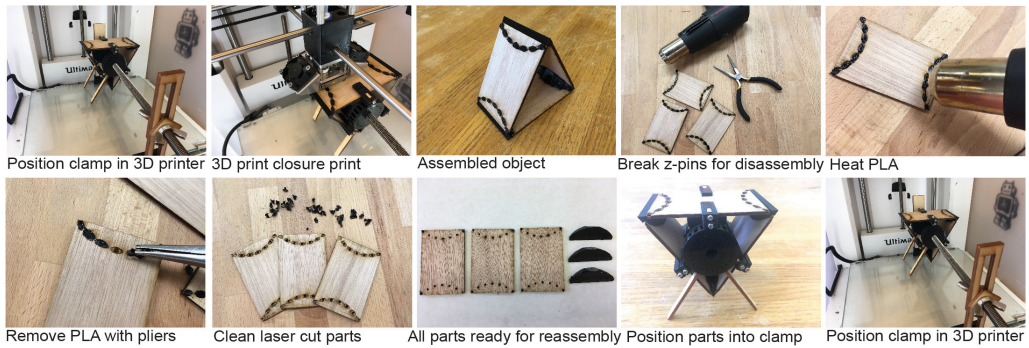
Figure 4.7. Assembly, disassembly and reassembly of the prism
