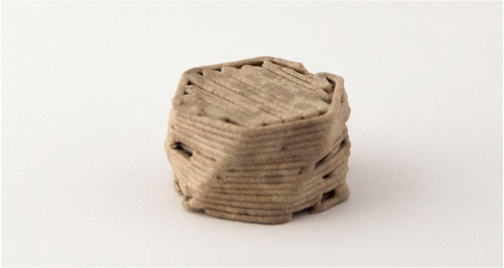
Figure 5.4. Result of material extrusion with recycled material.
