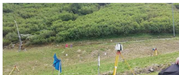
Figure 5: Scan location at Rumsoppen of the time series-based classification assignment. The location in the image is scanned 11 times at 10' interval. Trees and a piece of cloth are expected to be moved by wind.
