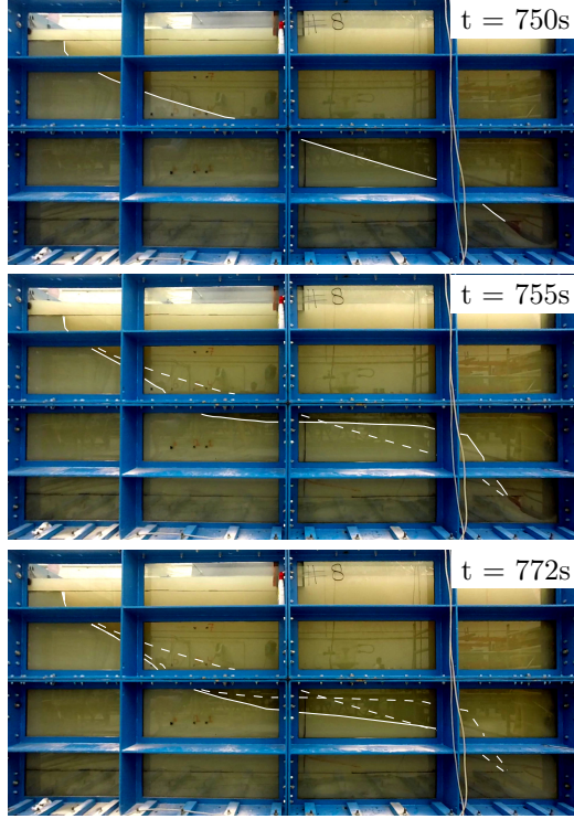
Figure 3.7: A Liquefaction failure observed during experiment 8.
