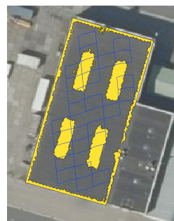
Figure 10. Example of a visualization obtained during the validation. Mapped ‘deviations’ are shown in yellow and can be overlaid with the (modified) pixels resulting from hyperspectral imagery pixels and contained in the building footprint (geometry in blue). Settings used: distance threshold 20 cm and angular threshold 2°.
