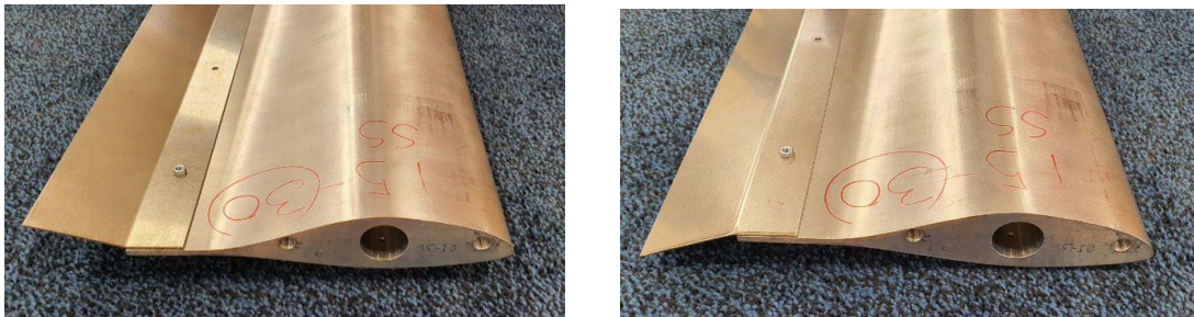
Figure 3: One of the DU models showing a 20 deg. negative (left) and positive (right) trailing edge (flap) angle when the airfoil faces the incoming flow with the thickest surface (negative angles).
