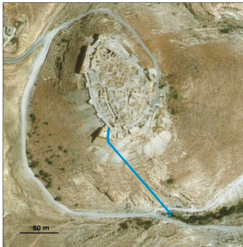
Figure 18. Shobak castle and itinerary of the subterranean spring. The subterranean spring is reached from inside the SW corner of the walls through a tunnel 50 m deep, and Ain Al Ragaye emerges at the foothills 170 m south [60].
