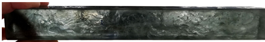
Fig. 7 “Lead CRT, 870 °C” specimen containing intense cord (seen as wavy lines) and bubbles
