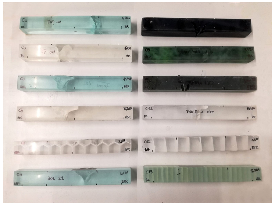
Fig. 27 Side view of kiln-cast specimens fractured during the 2nd series of four-point bending tests. Note that the primary crack starts perpendicular to the beam's long axis and then splits in the case of medium/large accumulated elastic energy (prior to cracking), or propagates as one crack in the case of low energy (e.g. crystallized specimens). At the top (compressive zone), the crack forms compression curls
